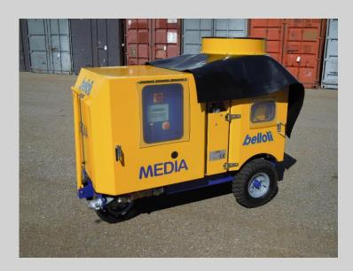
Pump for the application of dry- and wet-shotcrete and the pneumatical transport of fine gravel
